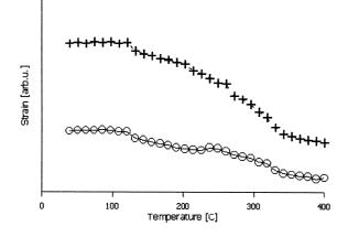
Fig. 2. Plot of strain changes in course of heating from  $25^{\circ}$  C to  $400^{\circ}$  C of Al<sub>x</sub>Ga<sub>1-x</sub>As/GaAs with x=04,3 implanted with 170 keV He<sup>+</sup> ions to the dose  $3\times10^{16}$  cm<sup>-2</sup> presenting the strain in mostly deformed layer (crosses) and the strain close to the surface (circles).
