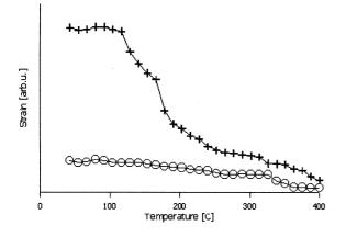
Fig. 1. Plot of strain changes in course of heating from  $25^{\circ}$  C to  $400^{\circ}$  C of GaAs implanted with 90 keV H<sup>+</sup> ions to the dose  $3 \times 10^{16}$  cm<sup>-2</sup> presenting the strain in mostly deformed layer (crosses) and the strain close to the surface (circles).
