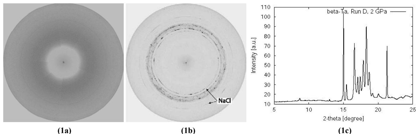
Fig. 1. Raw diffraction patterns, (1a) recorded in **Run F**, (1b) in **Run D**. A typical 1D powder diagram is given in (1c).
