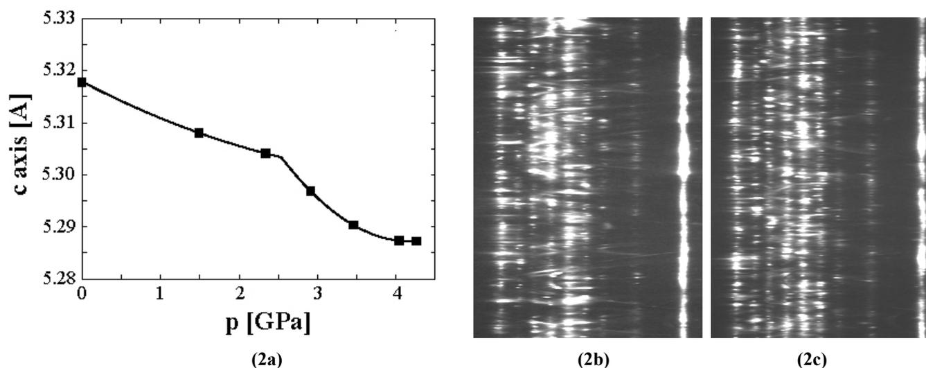
Fig. 2. The evolution of the  $c$  lattice parameter is given in (2a). Azimuthal representations of the raw images collected at 2.3 GPa (2b) and 3.4 GPa (2c) showing a stronger streaking effect just before the transition. The vertical axis is the azimuthal angle, while horizontal one corresponds to  $2\theta$ .
