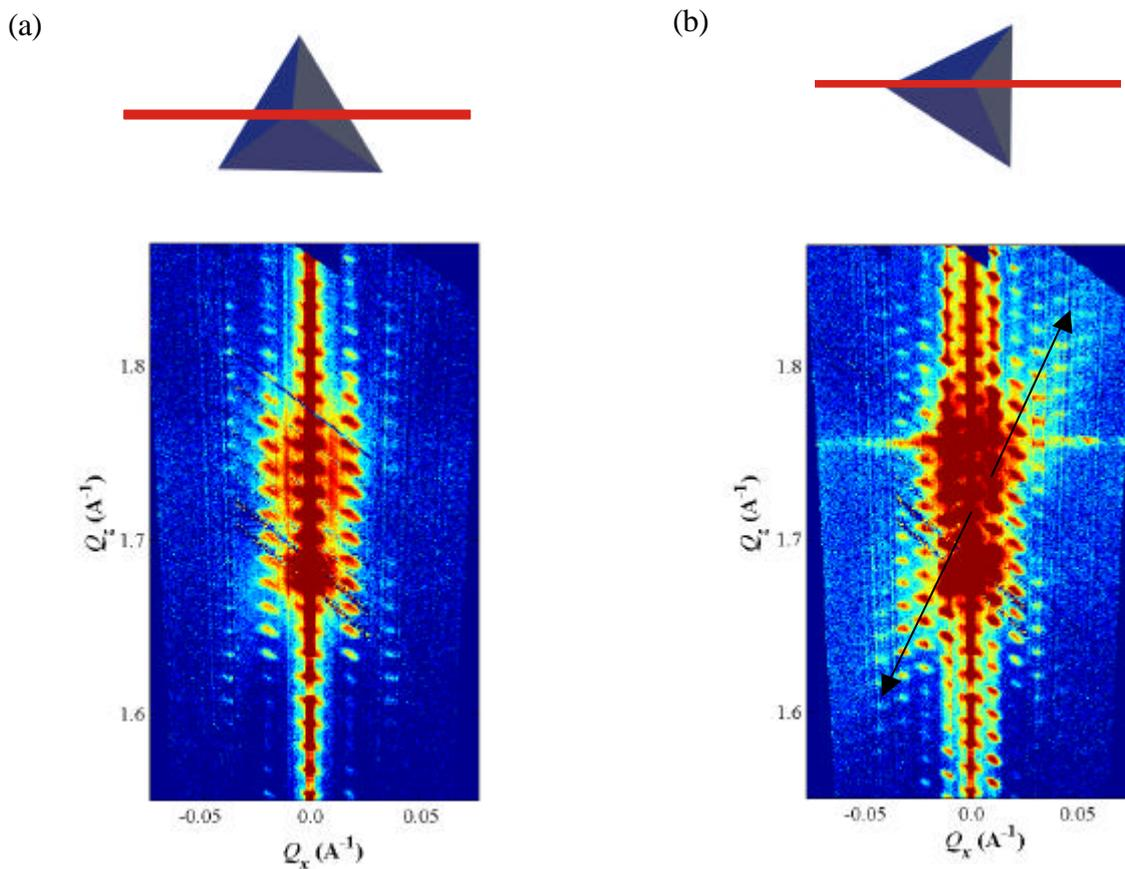
Figure 1 (a): Symmetric  $q_{\perp}$ - $q_{\parallel}$  reciprocal space map across the specular (111) reflection from a PbSe/ $Pb_{0.92}Eu_{0.08}Te$  quantum dot superlattice. No asymmetry due to facet truncation rods can be seen
