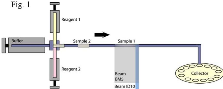
**Figure 1:** The new stopped flow apparatus. Two separate motors drive the syringes. One motor drives the reagents (1) and (2) for mixing. After waiting for a defined reaction time, the second drive pushes the sample across the beam and then into the collection tub
