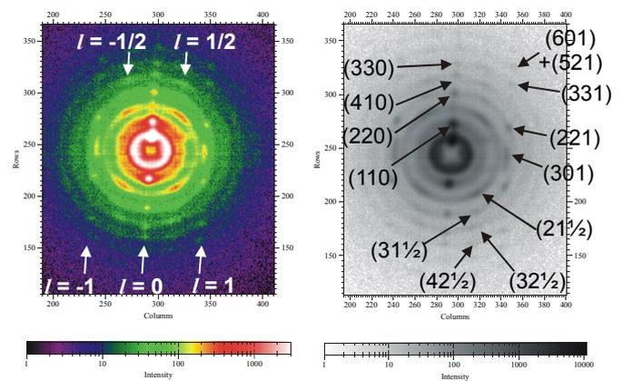
Fig.5. Diffraction pattern in colour and grey scale obtained from a dried 2D texture on a glass substrate after rotating by  $19.5^\circ$ . See text for further details.
