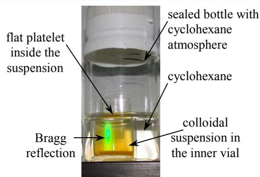
**Fig. 1(colour).** Green Bragg reflections of light from a depletion-induced colloidal crystal on a flat wall inside the
