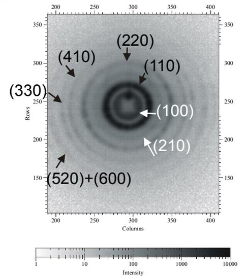
Fig.4. Diffraction pattern from a dried 2D texture on a glass substrate. Assignments to the Bragg circles are shown in black while the white arrows label rings originating from the Bragg cylinders.
