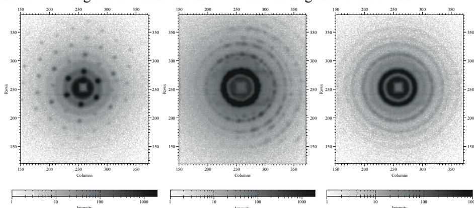
**Fig.2** Diffraction patterns from depletion-induced crystals at the wall of a flat capillary at three different positions.
