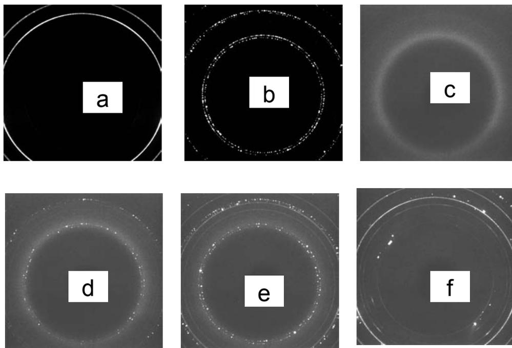
**Figure 3:** In situ melting and solidification experiment. a) XRD pattern of Cu pad, b) XRD pattern of Sn in solder paste, c) molten solder, d) crystalline structures appear shortly after melting, e) during solidification, f) PCB pad / solder interface after solidification.
