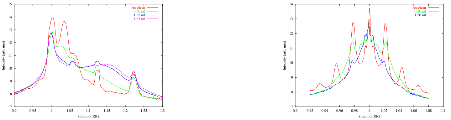
Figure 2: [left] k-scans along the (0 k 0.1) direction with respect to the Cr thickness. Note that the small bumps at k \sim 1.060 , 1.125 and 1.225 are always present on clean gold and likely belongs to residual disoriented crystallites. [right] hkscans around the (0 1 l) rod at l=0.12 for different Cr deposits.
