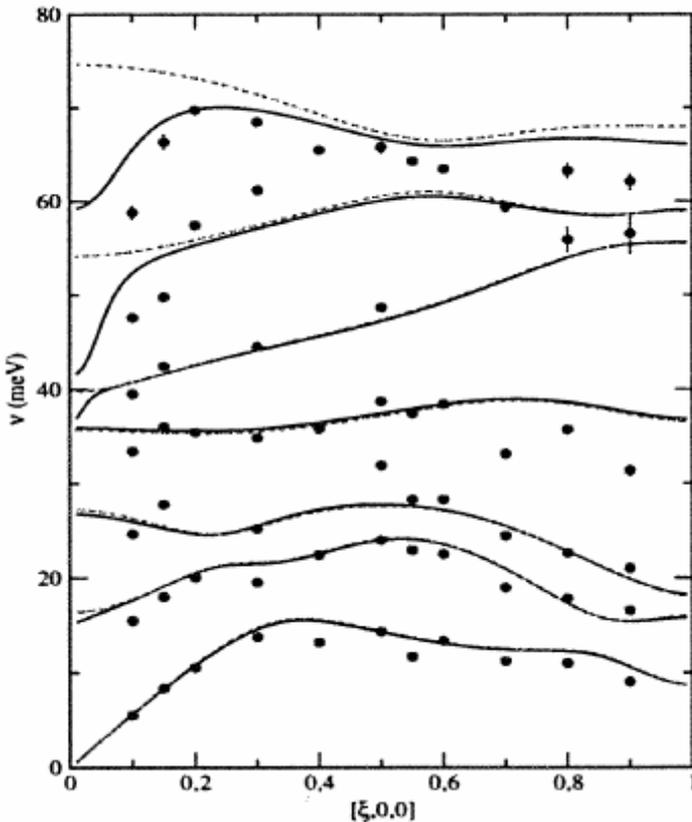
**Fig. 2** The dispersion of the longitudinal phonons in  $\text{Nd}_{1.98}\text{Ce}_{0.02}\text{CuO}_4$ . The solid and the dotted lines correspond to theoretical calculations for both an underdoped sample and the insulating compound  $\text{Nd}_2\text{CuO}_4$ . We see that there is an apparent anti-crossing of the two highest optical phonon modes near the zone center.
