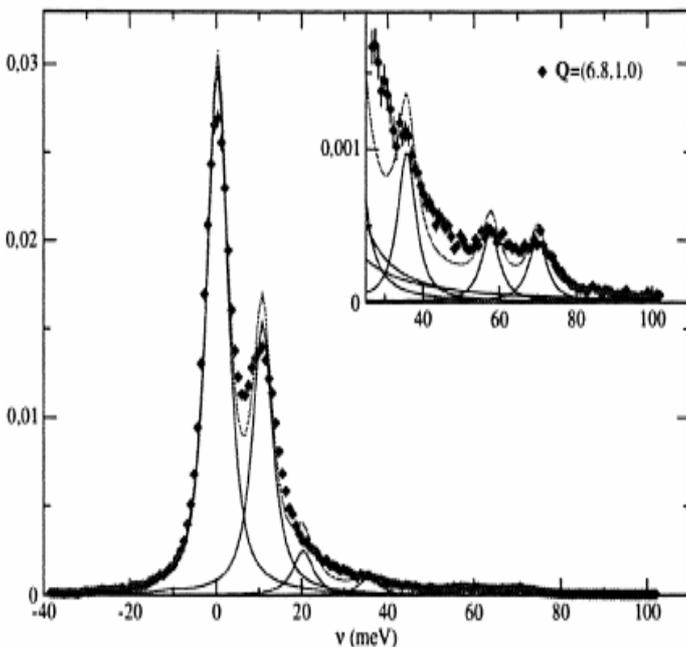
**Fig. 1** An energy scan at  $Q = (6.8 \ 1 \ 0) - q = (0.2 \ 0 \ 0)$  – for  $\text{Nd}_{1.98}\text{Ce}_{0.02}\text{CuO}_4$ . The resolution is determined by the  $\text{Si} (8 \ 8 \ 8)$  reflection. The largest peak is the elastic peak followed by the acoustic phonon mode. The continuous lines correspond to the fitting of the peaks where we have also taken into account the instrumental resolution. We also include a graph that shows the optical phonon modes under study.
