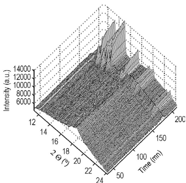
**Fig 2:** Time resolved WAXS pattern of CrAPO-5 crystallisation with a co-templated gel.
