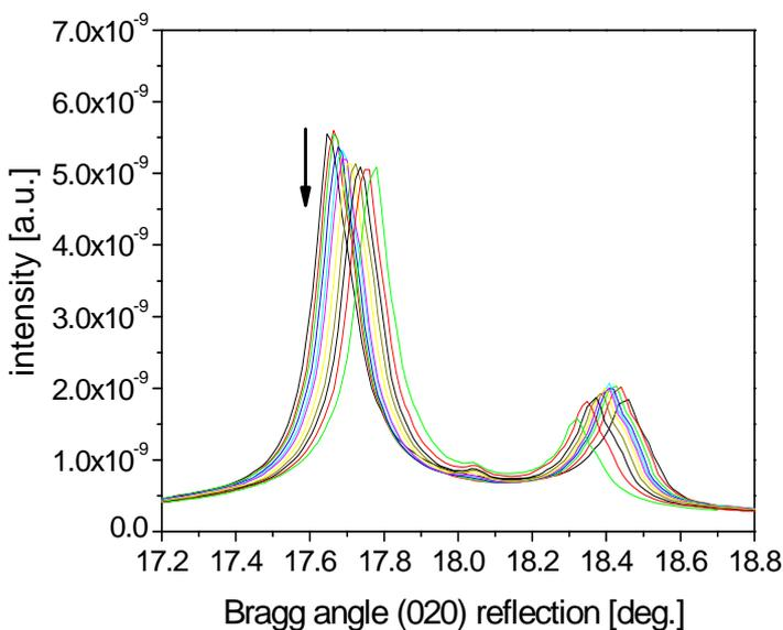
**Fig. 1:** Bragg profile of the BaTiO<sub>3</sub> crystal (020) reflection as function of temperature (30 °C for the outer peaks up to 110 °C for the inner peak). The <010> face was polarized predominantly perpendicular to the surface, so that the expected 1:2 ratio of long tetragonal to short tetragonal axis was inverted. The rising edge of the low angle peak was used to record scattering changes.
