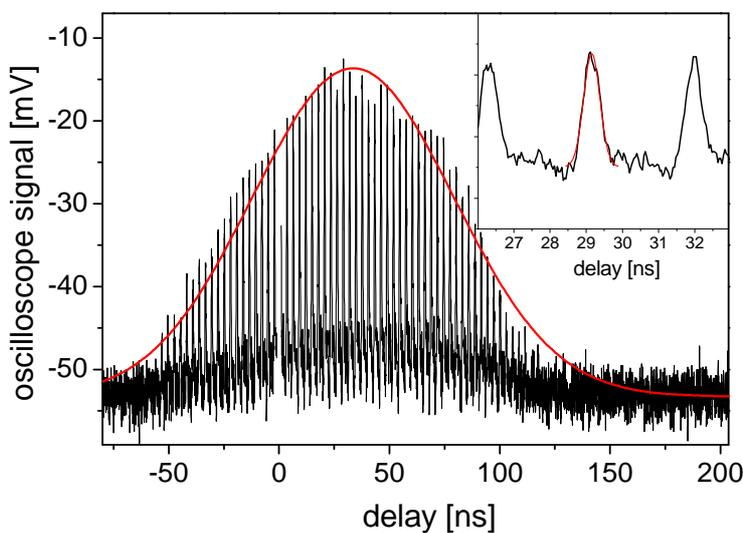
**Fig. 2:** Trace of the detector signal on the Tektronix oscilloscope in averaging mode for the pulses transmitted through the oscilloscope. The envelope of about 100ns represents the time resolution for integrating detectors. The inset is the enlargement of one peak, as recorded with an avalanche diode with pulse width of 450 ps FWHM.
