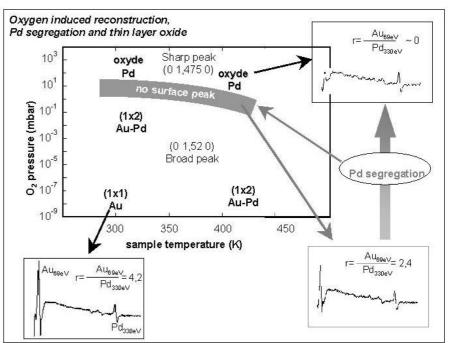
Just after the vanishing of the (1x2) LP (low pressure) reconstruction, the Auger ratio is equal to 2.4 showing a mixture of gold and palladium at surface. We also recorded data along several rods to analyse the (1x2) LP reconstruction. The quantitative analysis is under progress.
