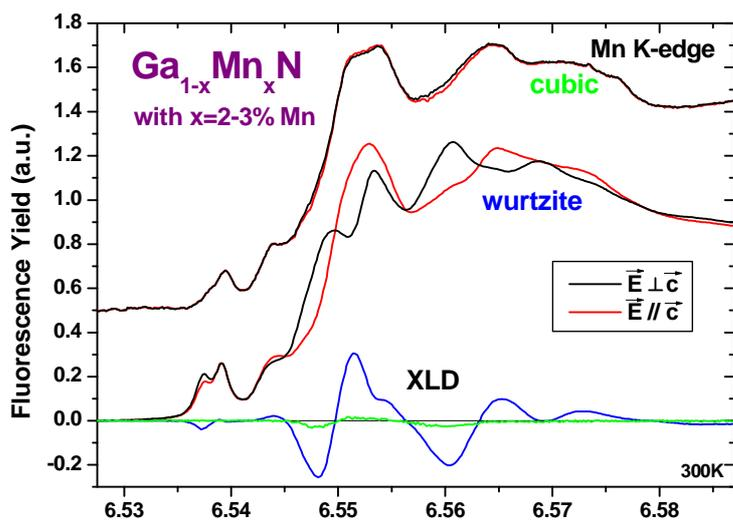
Fig.1 : X-ray Linear Dichroism recorded at the Mn K-edge at 300K in cubic (green colour) and wurtzite (blue colour)  $\text{Ga}_{1-x}\text{Mn}_x\text{N}$  with a equivalent Mn concentration  $x=2-3\%$ . The XANES spectra of both wurtzite and cubic samples have been normlized to an edge jump of unity for comparison.
