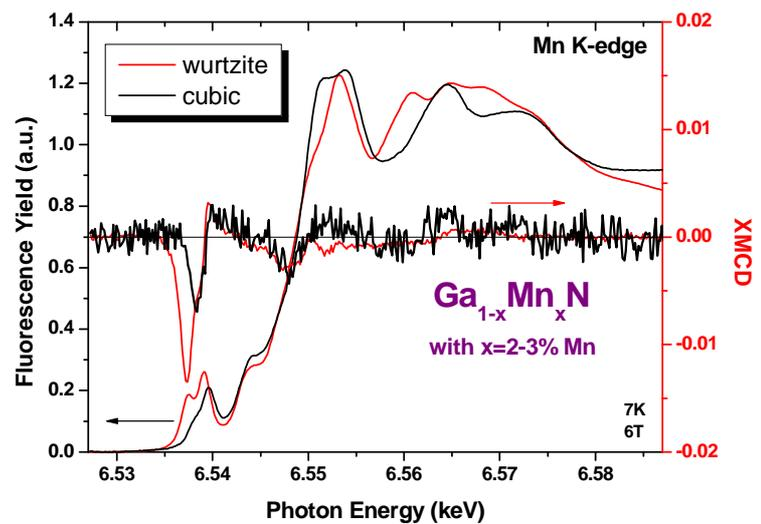
Fig.2 : X-ray Magnetic Circular Dichroism recorded at the Mn K-edge at 7K and under 6 Tesla external magnetic field in cubic (red colour) and wurtzite (black colour)  $\text{Ga}_{1-x}\text{Mn}_x\text{N}$  with a equivalent Mn concentration  $x=2-3\%$ .
