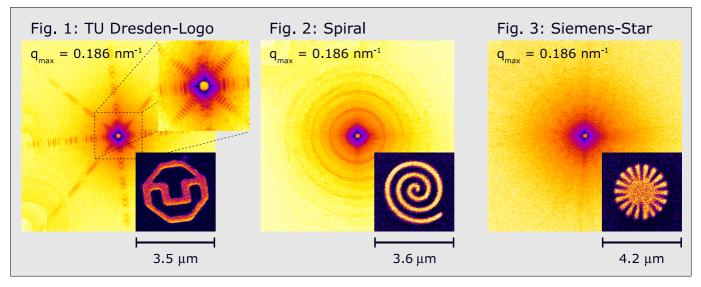
Fig. 1 shows that we could record a diffraction signal up to the edge of the detector giving a nominal resolution of 38 nm in x- and y-direction.
