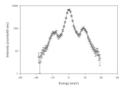
Fig. 1. Representative IXS spectrum of  $Fe_{0.94}O$  single crystal collected at 9.2 GPa. LA [110] phonon for Q(2.1;2.1;0).
