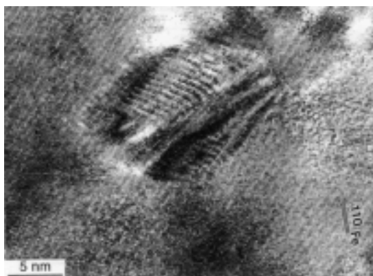
Fig. 1. HRTEM image of Cu precipitate in a complex alloy aged at 923 K for 1.8ks. [3]
