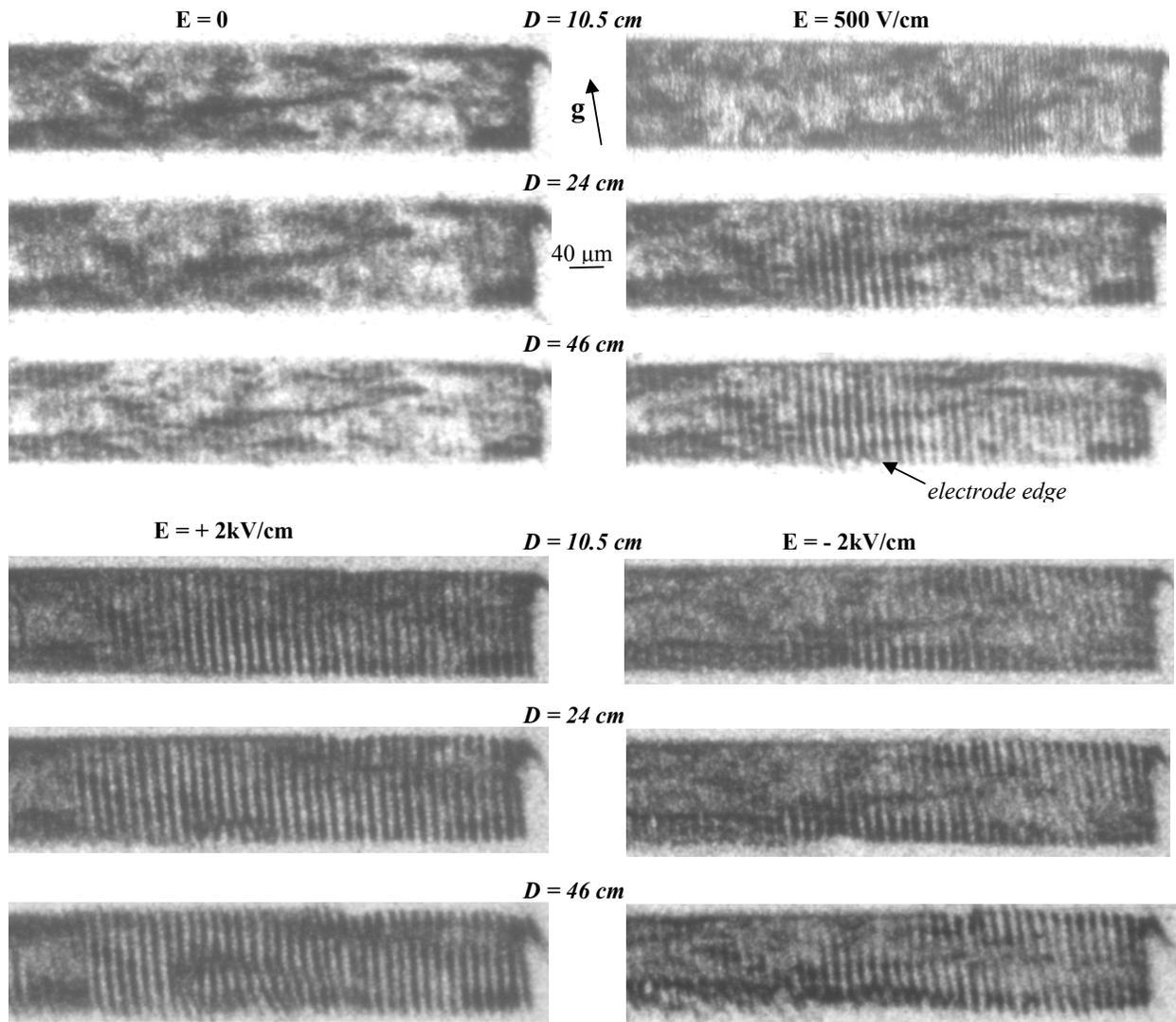
Figure shows a series of sections for the  $\bar{1}3\bar{1}$  reflection taken as a function of the sample-to-detector distance  $D$ , at various electrical fields  $E$ ,  $\lambda = 0.497\ \text{\AA}$ , period of poling =  $23\ \mu\text{m}$ .
