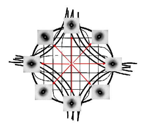
Model of principal, depth-averaged, collagen orientations in the human cornea (black lines). Microfocus WAXS data was collected at  $25\mu$ m intervals along 8 corneal meridians (red arrows). Limbal (radius = 5mm) WAXS patterns are shown.
