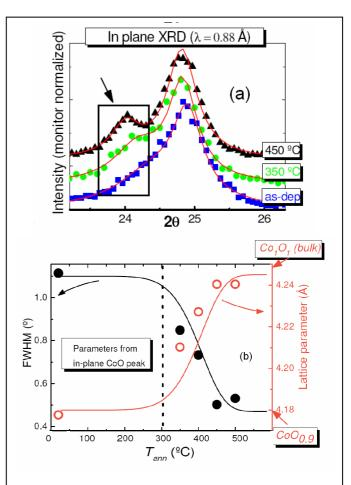
**Figure 2**. (a) in-plane x-ray diffraction for selected values of  $T_{ann}$ . taken using synchrotron radiation. The arrow indicates the CoO (002) signal. (b) shows the evolution of FWHM and lattice parameter with  $T_{ann}$  as extracted from the fits in (a)
