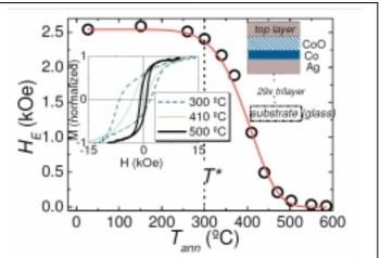
**Figure 1.** Post-deposition annealing (at temperatures  $T_{ann}$ ) dependence of the EB field, measured at 80 K. Insets: (left) corresponding hysteresis curves for selected values of  $T_{ann}$  and (right) the multilayer structure of the *as-deposited* sample, comprising essentially Co-CoO bilayers (30 in total) separated by Ag layers, and with an Ag capping (top) layer.
