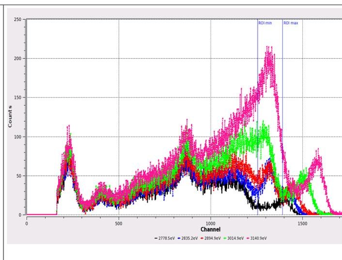
Figure 2: fluorescence spectra recorded by the energy-resolved detector as a function of incoming energy. ROI min and ROI max mark the fluorescence energy band of Cl. The raman contribution is clearly visible as well as its shift toward energy with incoming energy.
