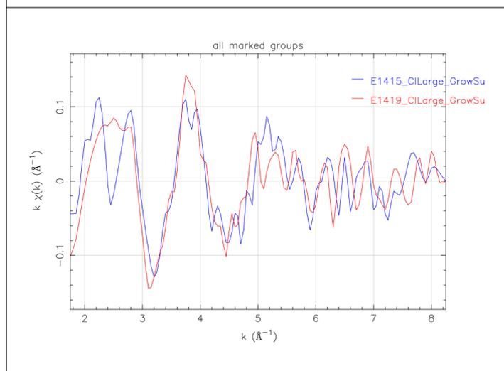
Figure 3: comparison between E1415 and E1419 exafs oscillations.
