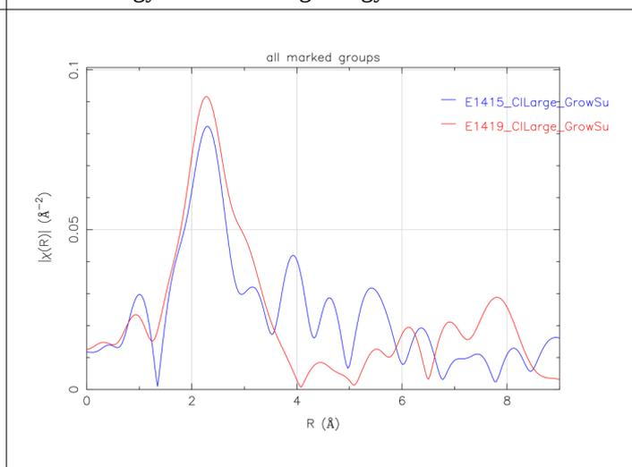
Figure 4: comparison between E1415 and E1419 Fourier transformed exafs oscillations.
