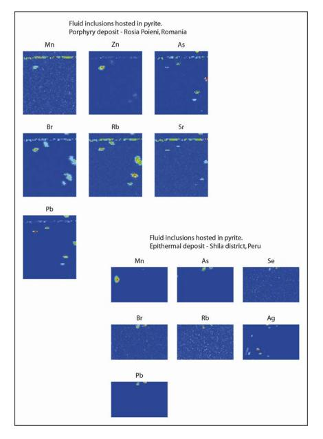
Quantitative results are still under processing, however, these first results demonstrate that ID18F standard setup allows analysis of fluid inclusions hosted in opaque minerals, thus offering a method for estimating fluid compositions directly in ore minerals.
