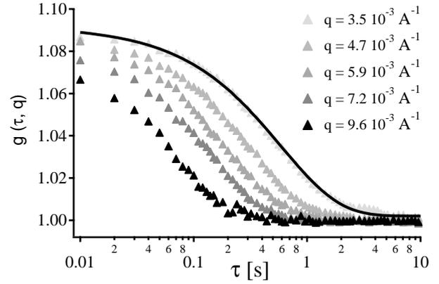
Figure 1: Raw correlation functions (symbols) for 2 vol% isotropic suspension of goethite. The solid black line is a fit by a stretched exponential function with  $\beta=0.85$ .
