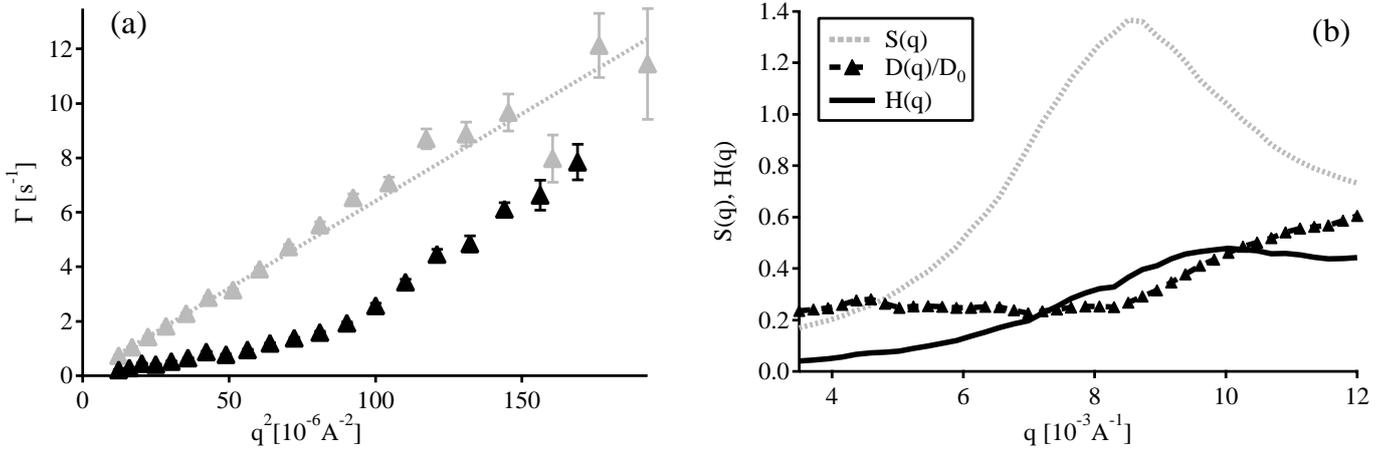
Figure 2: (a) Dispersion relations for a 2% isotropic goethite suspension (grey triangles), and a 6.7% nematic suspension (black triangles). The broken grey line is a fit constrained to go through the origin, that gives  $D_0 = 6.4 \cdot 10^{-16} \text{ m}^2\text{s}^{-1}$ . (b) Normalized diffusion coefficient (grey triangles), static structure factor  $S(q)$  (grey line) and hydrodynamic function  $H(q)$  (black line) of nematic phase, with  $q$  perpendicular to the nematic director.
