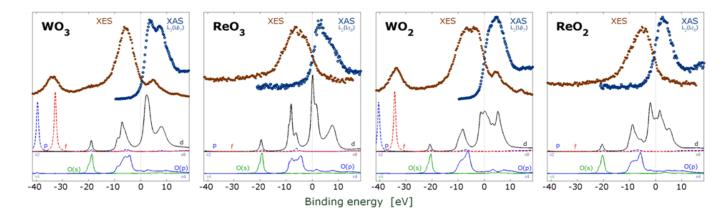
Fiure. 2.  $L\beta_{sat}$  &  $L\gamma$  emission and high resolution fluorescence detected  $L_{2,3}$  absorption spectra of WO<sub>3</sub>, ReO<sub>3</sub>, WO<sub>2</sub>, and ReO<sub>2</sub> powder samples compared with DOS calculations.
