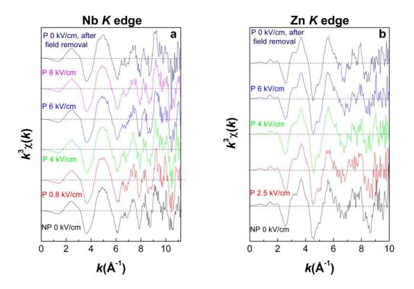
Figure 1 | EXAFS spectra of PbZn<sub>1/3</sub>Nb<sub>2/3</sub>O<sub>3</sub> perovskite as a function of the electric field. a, Nb K edge spectra b, Zn K edge spectra. NP and P accounts for Non Poled and Poled State
