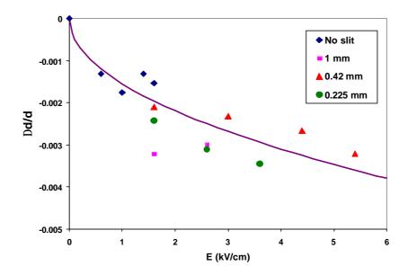
**Figure 4.** Relative changes,  $\Delta d/d$ , of the (220)-d-spacing in the light-irradiated CZT crystal (S5,  $I = 530 \text{ mW/cm}^2$ ), as a function of the applied electric field, E (in kV/cm). Measurements were performed with different slits, which limited the irradiated area: blue diamonds – no slit; pink squares – 1 mm; red triangles – 0.42 mm; green circles – 0.225 mm.
