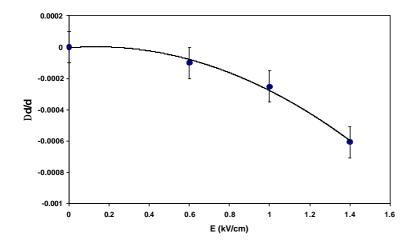
**Figure 3.** Relative changes,  $\Delta d/d$ , of the (111)-*d*-spacing in the light-irradiated CZT crystal (S4,  $I = 530 \text{ mW/cm}^2$ ), as a function of the applied electric field (in kV/cm). Solid line represents best fit to parabolic function.
