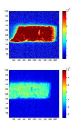
**Figure 1.** Diffraction images taken with a CZT crystal (S4, (220)-reflection) with no light and no electric field (upper panel) and under light irradiation and electric field application (lower panel:  $I = 530 \text{ mW/cm}^2$ , E = 1.4 kV/cm).
