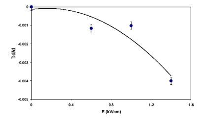
**Figure 2.** Relative changes,  $\Delta d/d$ , of the (220)-*d*-spacing in the light-irradiated CZT crystal (S4,  $I = 530 \text{ mW/cm}^2$ ), as a function of the applied electric field (in kV/cm). Solid line represents best fit to parabolic function.
