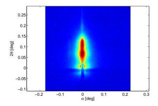
During the wetting process, the GISAXS map does not change in shape, but only in intensity, indicating that there is the absence of nanometric superhydrophobicity.
