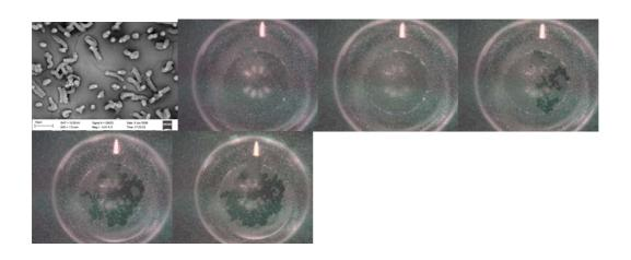
In Fig.1 we report a SEM image of a sample (photo a) and a typical time evolution of the wet area (dark regions) as seen by the digital microscope.
