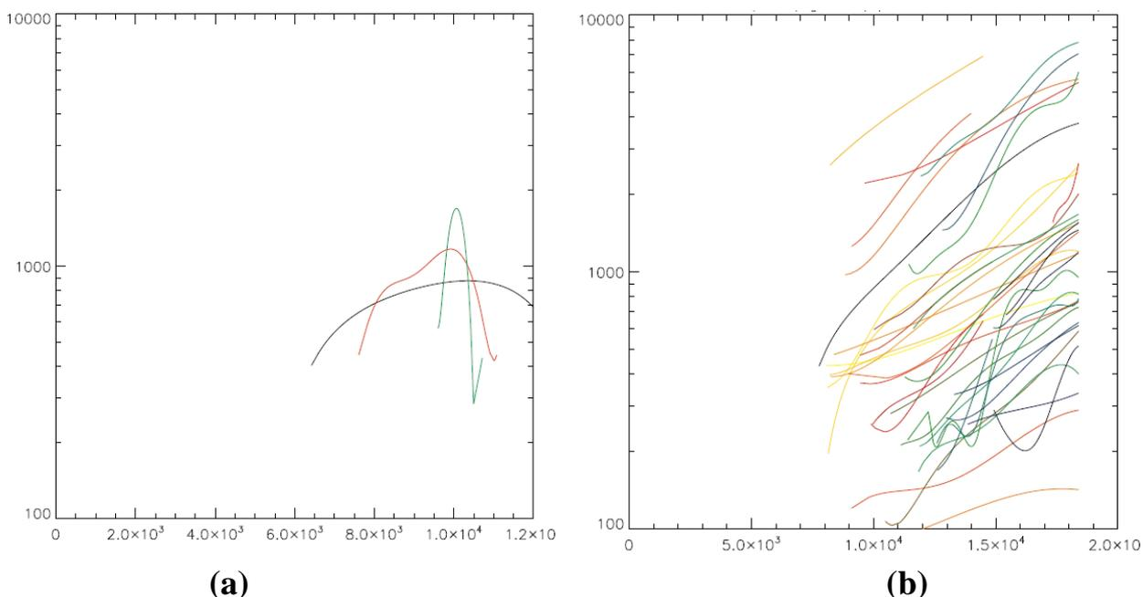
Fig. 1 Evlution of the diffracton intensity (vertical axis) of individual recrystallizd grains as a function of annealing time (horrorizal axis) to show the influence of ECAP temperature on the recrystallization behavior of CP-Ti. (a) sample ECAP-4P@450°C, during annealing at 485°C , (b) sample ECAP-6P@350°C , during annealing at 450°C .
