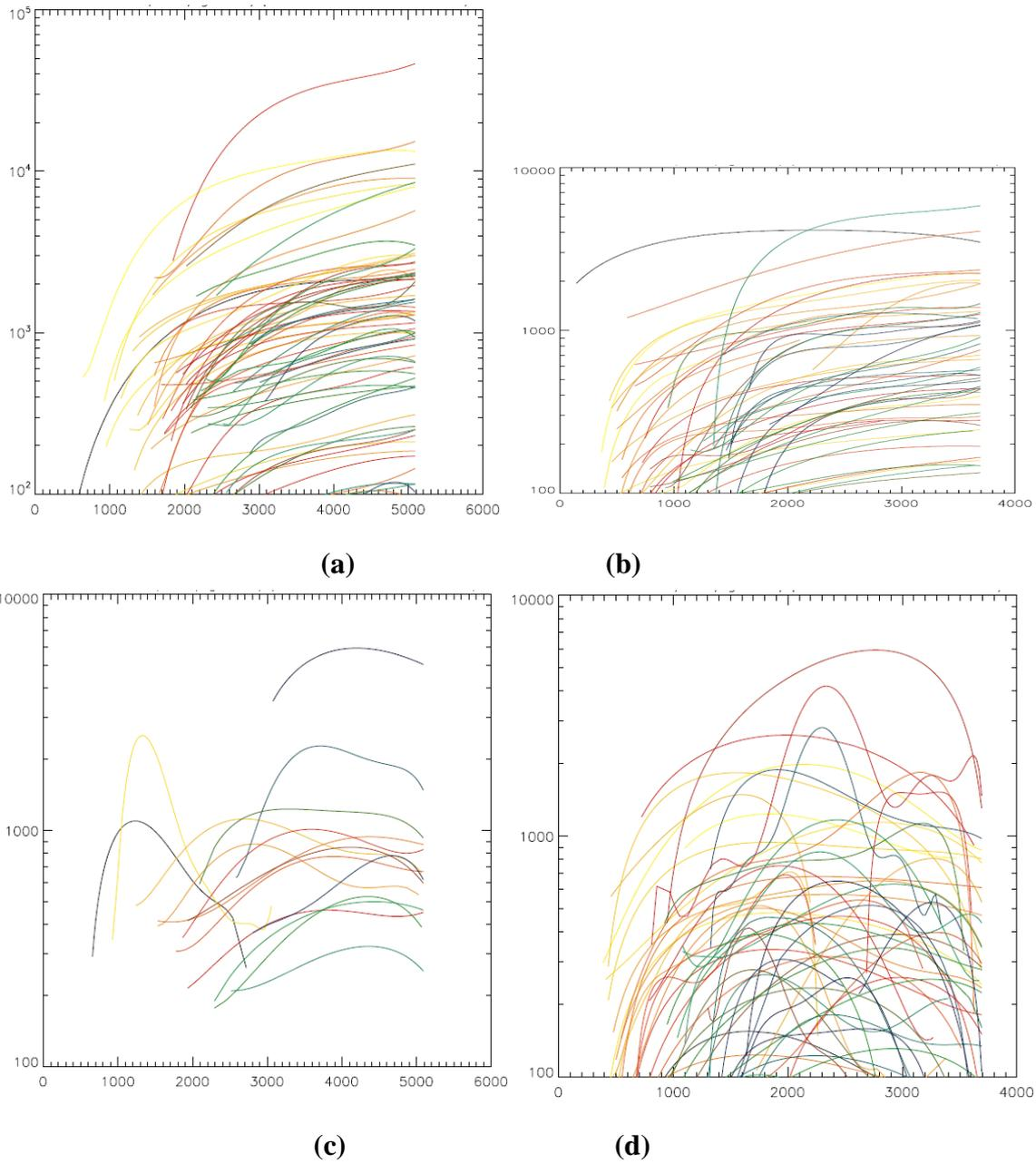
Fig. 2 The growth curves of individual recrystallized grains during during isothermal annealing at 525 °C. (a), (c) sample ECAP-4P@450°C; (b), (d) sample ECAP-8P@450°C
