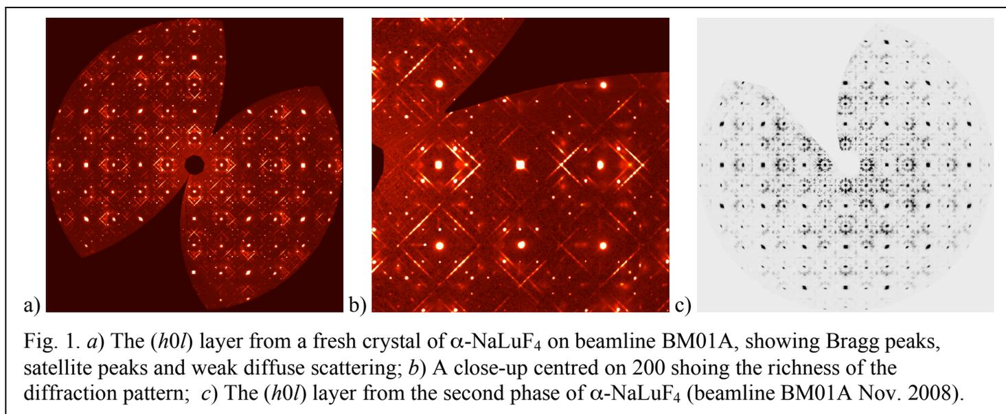
Fig. 1. *a)* The  $(h0l)$  layer from a fresh crystal of  $\alpha$ -NaLuF<sub>4</sub> on beamline BM01A, showing Bragg peaks, satellite peaks and weak diffuse scattering; *b)* A close-up centred on 200 showing the richness of the diffraction pattern; *c)* The  $(h0l)$  layer from the second phase of  $\alpha$ -NaLuF<sub>4</sub> (beamline BM01A Nov. 2008).
