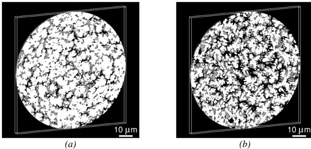
Figure 2. 0.6  $\mu\text{m}$  thick cylindrical cross sections of leached (a) Ni-75.0at%Al and (b) Ni-77.5at%Al powders produced by spray atomisation.
