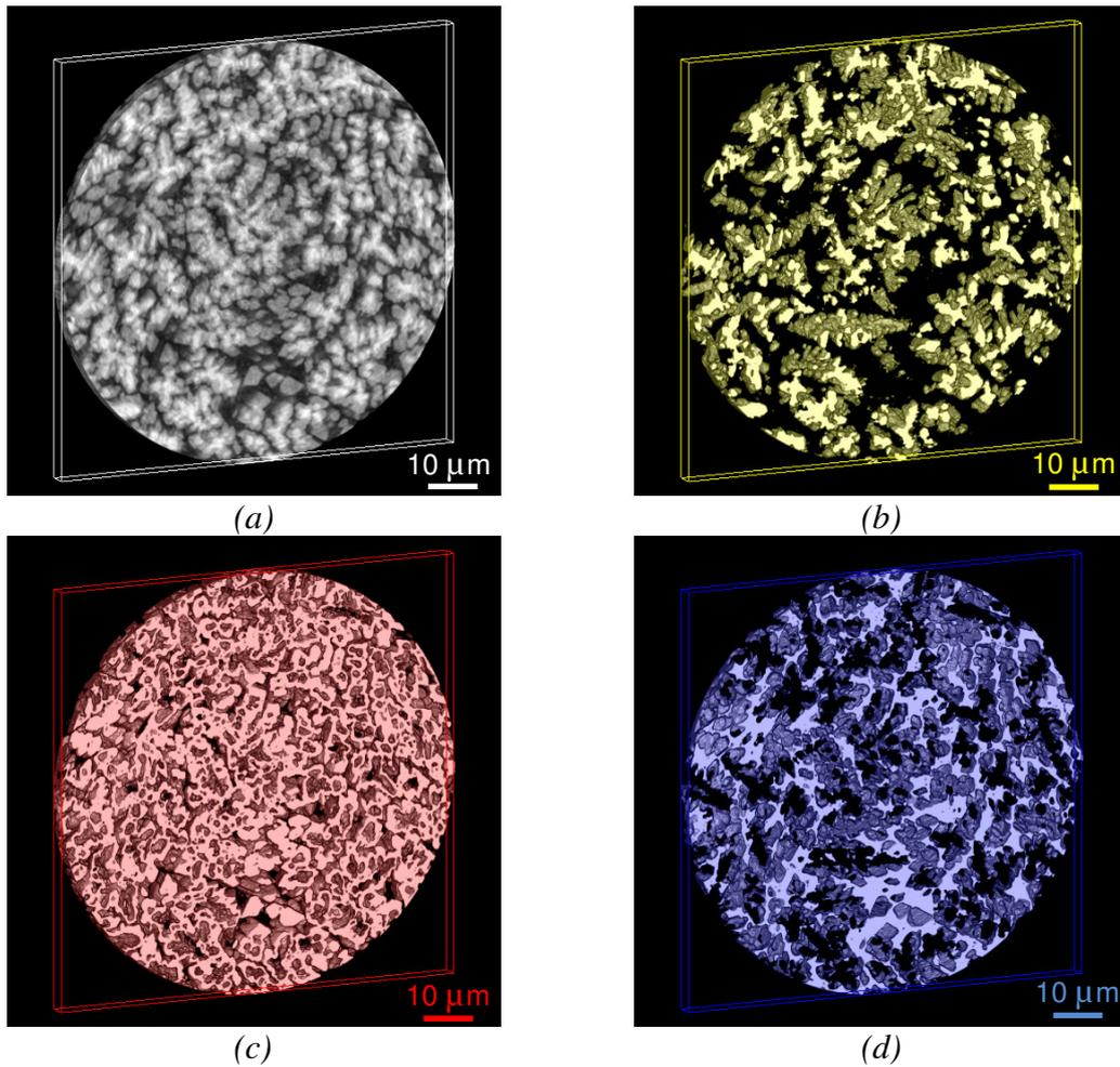
Figure 1. 1.2 μm thick cylindrical cross sections showing (a) the inner microstructure of a Ni-77.5at%Al droplet, (b), (c) and (d) 3D distribution of the  $\text{Ni}_2\text{Al}_3$ ,  $\text{NiAl}_3$ , and eutectic phases respectively.
