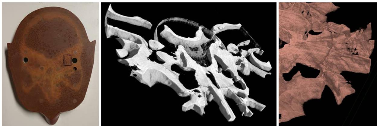
Figure 9. Picture of the Alderson-Rando Phantom (left), inner reconstructed volume (centre), particular of the reconstructed volume (right). This analysis was carried out with beam energy of 55 keV.
