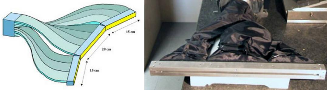
Figure 2 – Scheme and picture of the fiber optics fan. [1]
