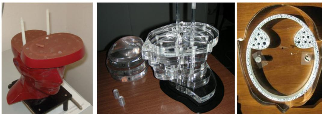
Figure 6 – Pictures of Alderson-Rando Phantom (left) and of the plexiglass phantom (centre) and the modified slice with enclosed a geometric hydroxylapatite insert.
