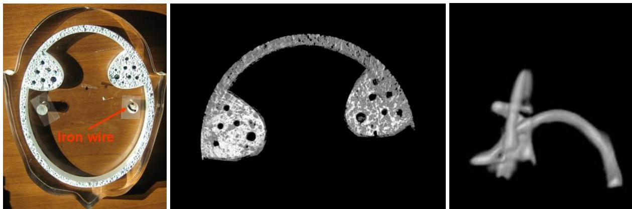
Figure 7. Picture of the plexiglass phantom (left), 3D volume reconstructed with binning 3 (centre), detail of the iron wire (right). This analysis was carried out with beam energy of 55 keV.
