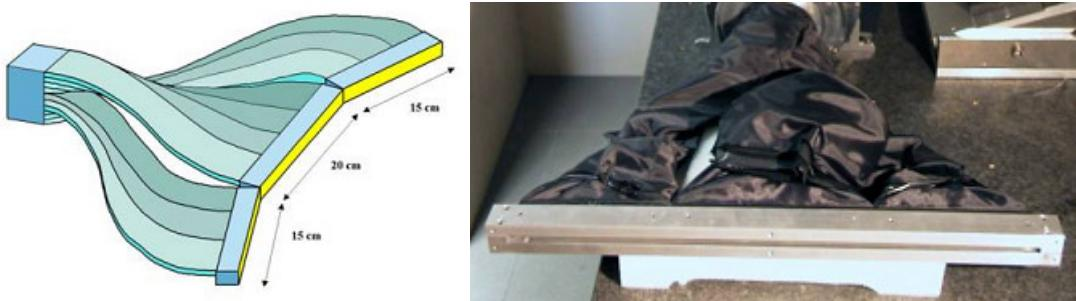
Figure 2 – Scheme and picture of the fiber optics fan. [1]
