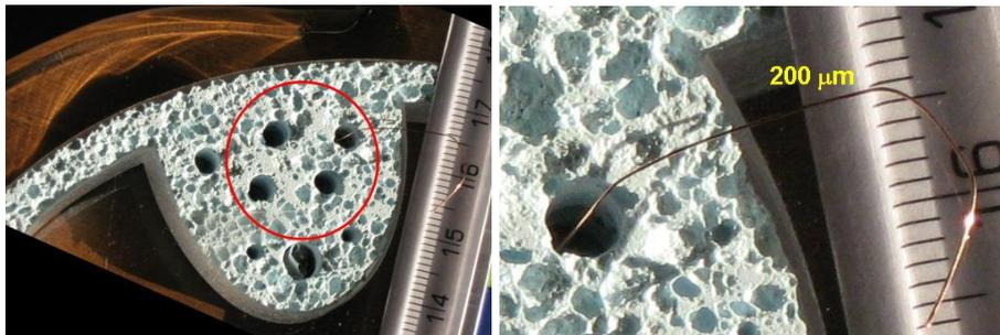
Figure 8 - Pictures of the region of interest studied with high resolution CT analysis (red circle, left), zoom of the hole where the copper wire (200  $\mu\text{m}$ ) is placed (right). This analysis was carried out with beam energy of 55 keV.
