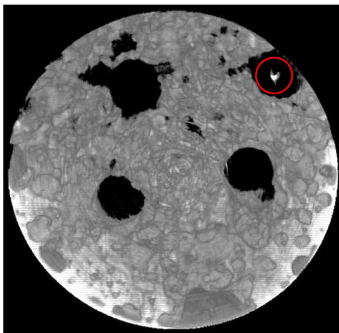
Figure 8. Reconstructed volume in local tomography at high resolution. See the copper wire with a diameter of 200  $\mu\text{m}$  (red circle) in a hole (diameter of 3 mm) bored in the hydroxyapatite layer.
