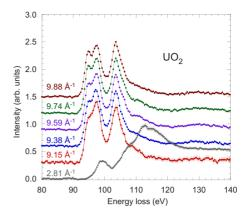
FIG. 2. (Color online) NIXS spectra measured for  $UO_2$  at the uranium  $O_{4,5}$  edges with a fixed final energy of 9.689 keV, at different values of the scattering vector q as indicated. The NIXS signal has been normalized to the peak centered at 104 eV in the high-q spectra.
