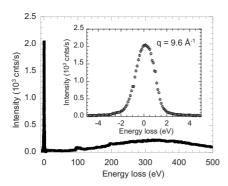
FIG. 1. Photon energy-loss spectrum measured for  $UO_2$  at room temperature over an extended energy range including the elastic and Compton peaks. Data have been collected with a fixed final energy of 9.689 keV, at a transferred wave vector q=9.6 Å<sup>-1</sup>. The inset shows the elastic peak, whose full width at half maximum is 1.3 eV.
