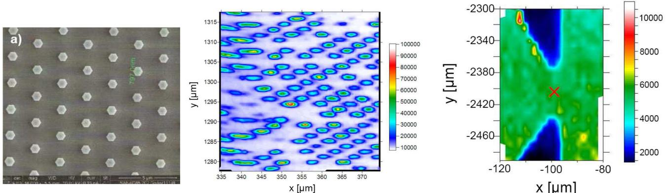
Fig. 1: a) Scanning electron micrograph and b) scanning X-ray diffraction map at the GaAs(111) Bragg peak of GaAs nanorods. c) Scanning absorption image of the AFM-tip.
