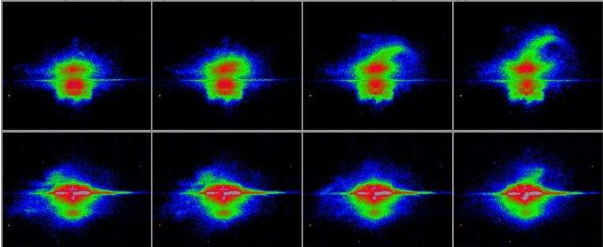
Fig. 2: Two sequences of XRD images taken at two different rocking angles during the compression of a single GaAs nanorod.
