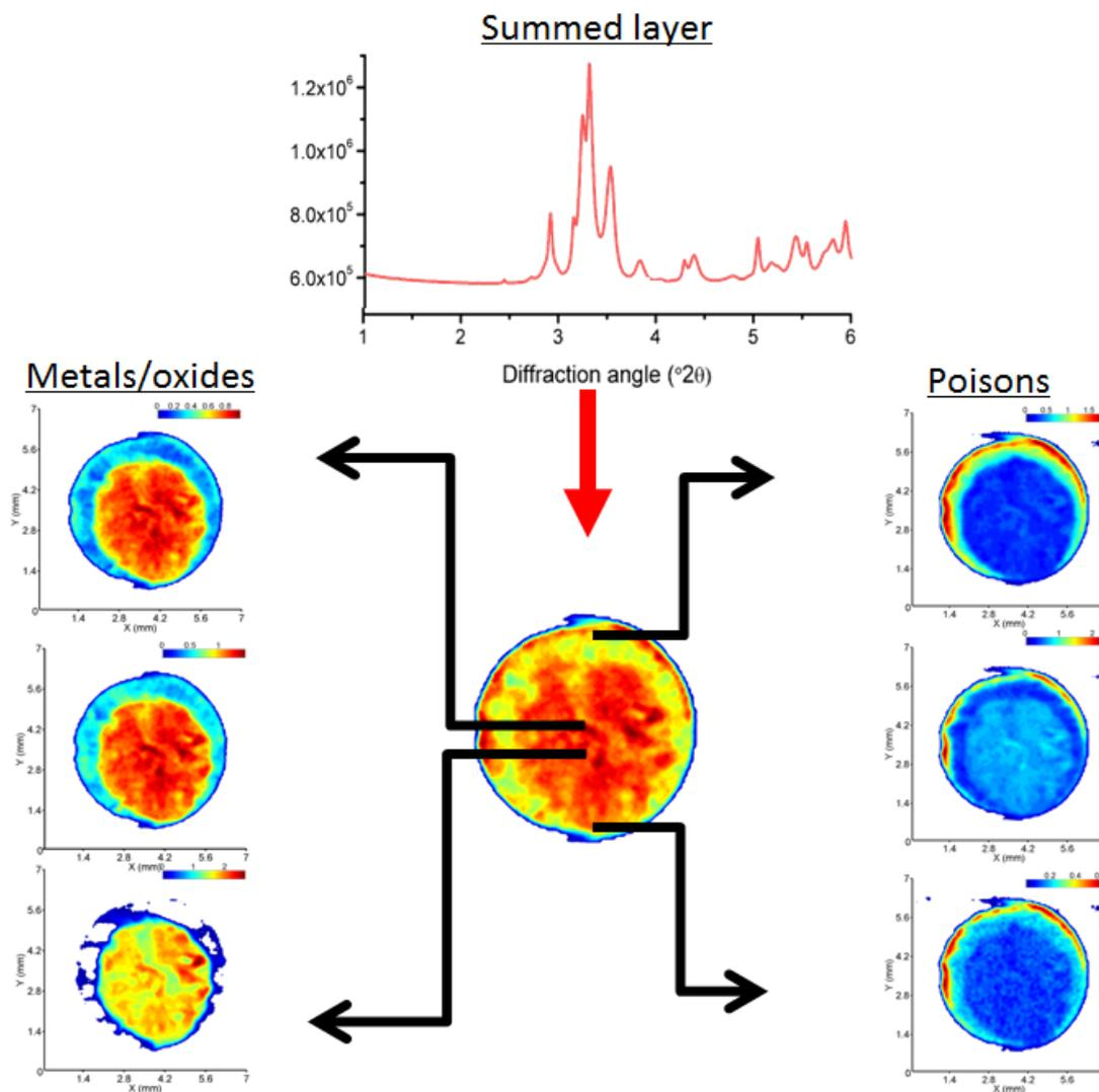
**Figure 1:** Demonstration of some of the data obtained from this beam time. The image shows how the spatial details from the summed diffraction image of the entire layer can be obtained using back projection algorithms, allowing us to observe the distribution of various metals, oxides and poisons within an cylindrical industrial catalyst body.
