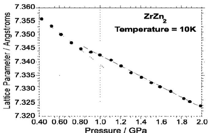
**Figure 1 – Pressure dependence of the lattice parameters for  $ZrZn_2$  at 10K obtained from high pressure, low temperature powder diffraction study at ESRF (ID09A).** Between 0.8 and 1.0 GPa there is a clear discontinuity in the lattice parameter. This corresponds to the pressure at which the ferromagnetic ordering temperature is suppressed at 10K with the corresponding observation of unusual power laws in resistivity data. (Lines are guide to the eye).
