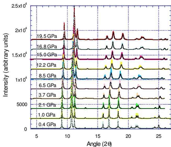
**Figure 2 – Powder diffraction data of  $ZrZn_2$  at 10 K at different pressures.** For each pressure curve the coloured lines are from the experimental data and the black lines are the fitted refinement using the GSAS software package.
