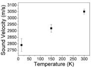
Fig. 3: Temperature dependence of the sound velocity in the 500 nm-wide Fe squares
