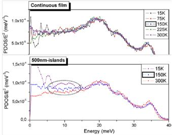
Fig.2: Temperature dependance of  $PDOS/E^2$  for the 500 nm-wide-Fe squares and for the continuous reference film.
