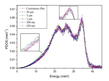
Fig. 1: Phonons densities of states of Fe squares of different lateral sizes compared with the ones of a continuous film, measured at 300K.
