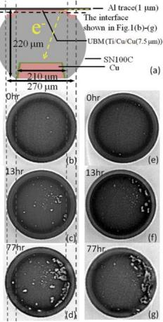
For comparison, Figure 3 shows the evolution of the interfaces of two unpowered solder bumps, which only suffered 130degC thermal aging. Compared to the image taken at 0hr, after 77hrs, there are also several small voids founded at the interface, which means the reaction between UBM and solder body can introduce
