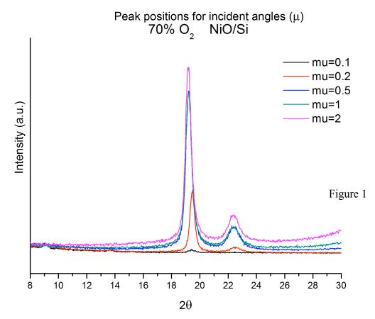
Figure 1 the diffraction pattern, obtained for the sample grown with 70% oxygen in the plasma, on a silicon substrate. There is a clear shift of the (111) peak towards higher angles as the incidence angle decreases, suggesting a change in the lattice constant as with depth: the lattice parameter would be higher closer to the interface.
