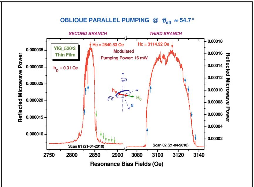
**Fig. 1** PP microwave absorption spectrum of a YIG thin film recorded using a special microwave TE<sub>102</sub> cavity designed to satisfy the requirement:  $\mathbf{h}_p \parallel \mathbf{H}_0 \perp \mathbf{N}$ . Note the superstructure of narrow exchange-driven spin waves resonances [3].
