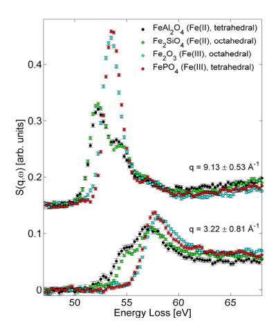
Figure 1: XRS spectra of the Fe  $M_{2/3}$ edge of differently coordinated Fe<sup>2+</sup> and Fe<sup>3+</sup> for low and high momentum transfer.
