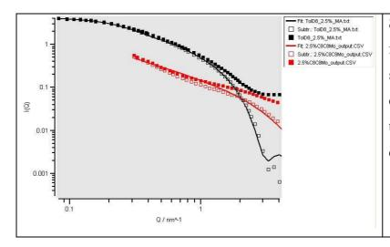
SAXS (red) and SANS (black and obtained from ILL-D22 experiment on similar samples) scattering raw (full) and corrected (empty) data) adjusted using a ribbon-like form factor taking into account packing parameter constrain with various contrast.
