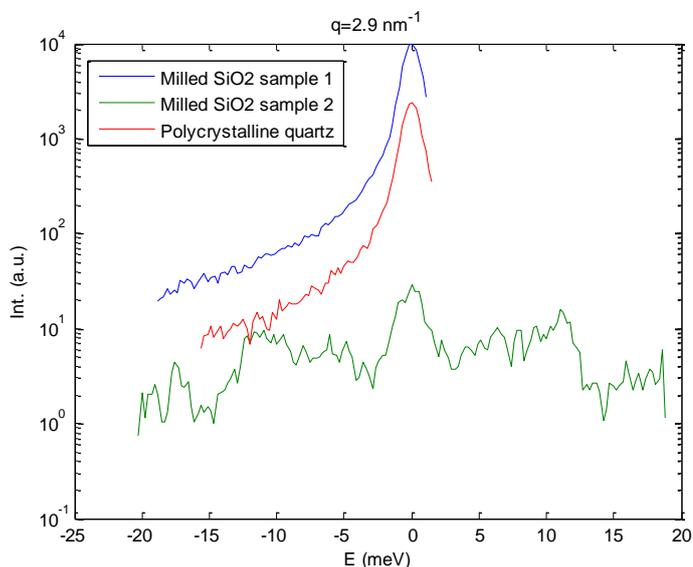
*Figure 1: IXS spectra collected at an exchanged wave-vector  $q=2.9 \text{ nm}^{-1}$  on two compacted pellets with nanometer sized grains and polycrystalline quartz with micrometer size grains.*
