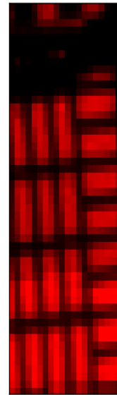
Fig. 2 Elemental map (Pt L\alpha line) of the sample surface used to select the capacitor to investigate. The single capacitor dimensions are 300 \times 800 \mu\text{m}^2 .
