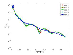
To avoid beam damage of the OTS layer, the sample was shifted horizontally after each reflectivity curve. Thus, we checked first the homogeneity of our samples. The Figure on the left shows reflectivity curves from 4 different spots on an OTS-coated silicon wafer immerged in water. From this figure, it can be seen that the sample is homogeneous and that the OTS layer is destroyed if a second reflectivity is measured on the same spot.
