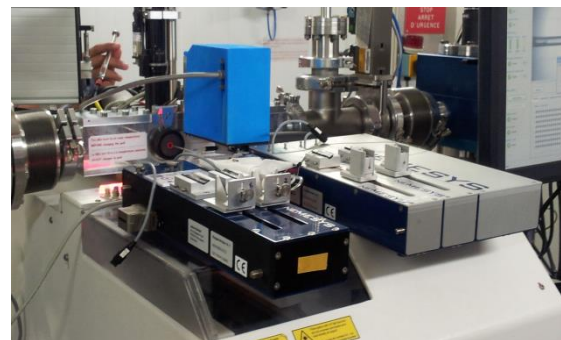
Figure 1- schematic design of chip connected to BM 29 pod (left) ; 4 syringe pumps are connected to chip to generate circulating droplets of aqueous solution in continuous circulating oil (right)
