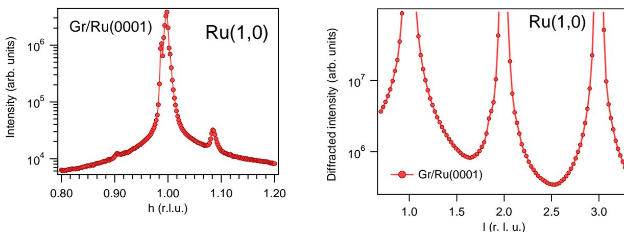
**Fig.1** GR/Ru(0001) : left) in-plane scan measured along the  $h$  direction in the neighborhood of the (01) CTR of Ru at  $l=0.2$  r.l.u.; right) Ru(1,0) CTR ( $lhkl = 1,0,l$ )
