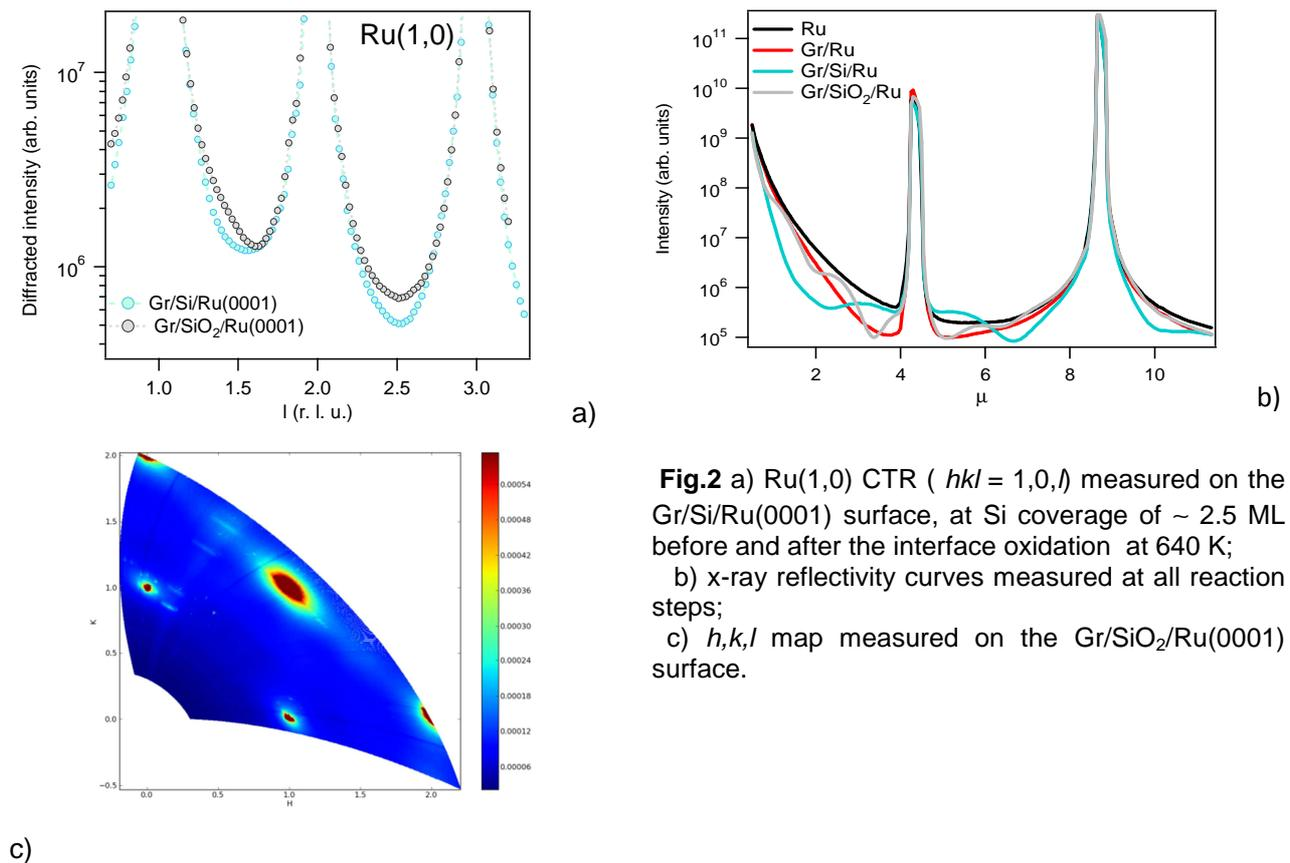
**Fig.2** a) Ru(1,0) CTR ( $hkl = 1,0,l$ ) measured on the Gr/Si/Ru(0001) surface, at Si coverage of  $\sim 2.5$  ML before and after the interface oxidation at 640 K;
