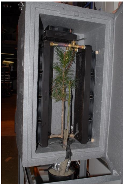
Fig.2 Freeze box designed for freezing a complete tree without freezing the root system. Samples (here Pinus sylvestris ) were then quickly transported for image acquisition.
