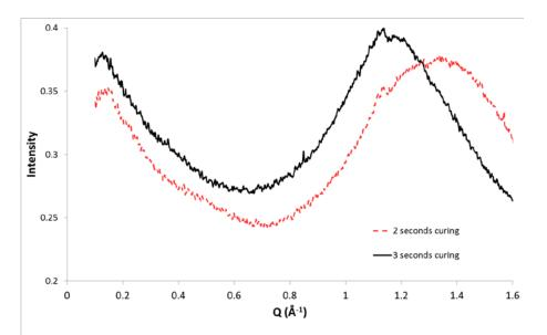
**Figure 2**: 60% wt hydrogenous Bis-GMA and 40% wt TEGDMA with 0.1 Camphorquinone photo-initiator. The broken (red) and solid (black) curve shows the structure after photo-curing for 2 and 3 seconds respectively.
