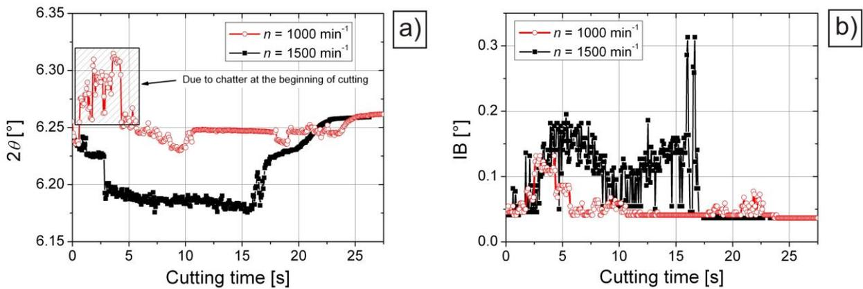
**Figure 2:** Evolution in time for the  $2\theta$  value (a) and integral width IB (b) for the 311 peak of aluminium during the cutting process.
