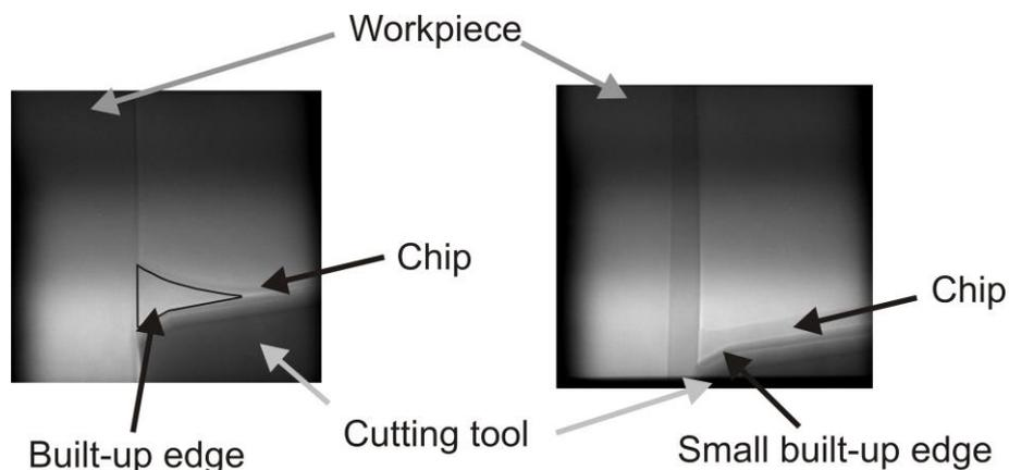
**Figure 3:** Radiographic images of built-up edge formation of aluminium for  $n = 1000 \text{ min}^{-1}$  (left: very large and stable BUE outlined in black) and  $n = 1500 \text{ min}^{-1}$  (right: negligible instable BUE).
