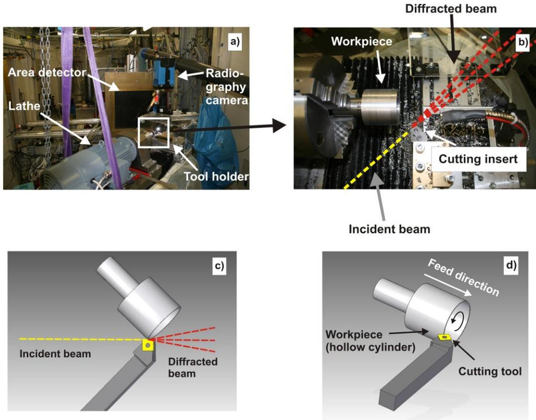
**Figure 1:** Documentation of orthogonal metal cutting operation in measurement hutch of ESRF beamline ID 15A (a) and b)). The lathe, detectors, workpiece, cutting tool and the optical paths of the incident and the diffracted beam are indicated. In the second row (c) and d)) the schematic setup is shown with drawing of workpiece and tool.
