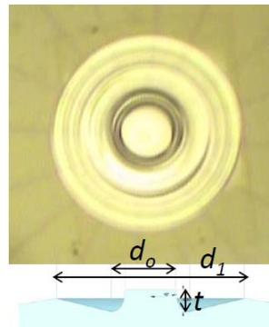
**Fig. 1** : Geometry of the tores machined in the diamond anvil.  $d_0=16 \mu\text{m}$  for all runs, see **Table 1** for  $d_1$  and  $t$ .
