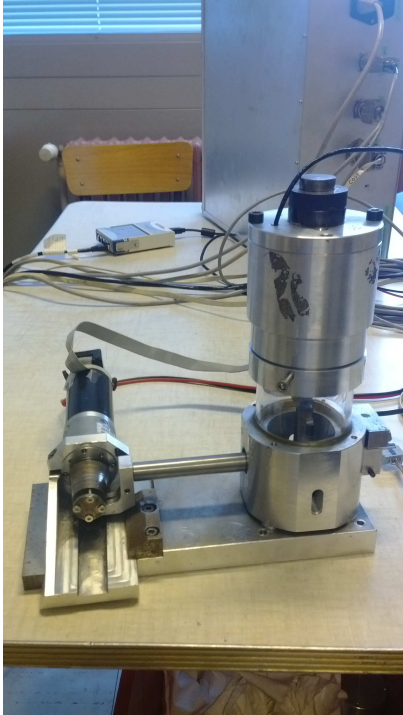
Fig. 1: In situ fatigue machine used during experiment MA2184.
