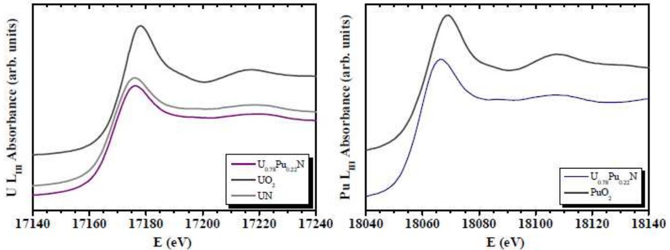
Fig 1 XANES spectra of damaged  $U_{0.78}Pu_{0.22}N$  NIMPHE fuel at  $U L_{III}$  and  $Pu L_{III}$  edges (The XANES spectra of UN,  $UO_2$  and  $PuO_2$  are presented as reference materials).
